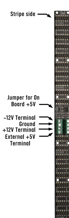
If you plan on using an external +5V source, like from your power supply, DO NOT POPULATE THE +5V JUMPER! It will cause damage to your equipment.
